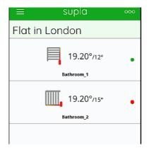
If a heater in the App has a red dot to the right, make sure that it is powered and switched on, and that it has an internet connection. Try restarting both the heater and the modem.
