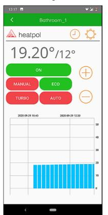
The first temperature ( $19.20^{\circ}$ C) - is measured with the remote / temp. sensor (H+R). This is the actual room temperature. The second ( $12^{\circ}$ C) is the temperature set for the room.
